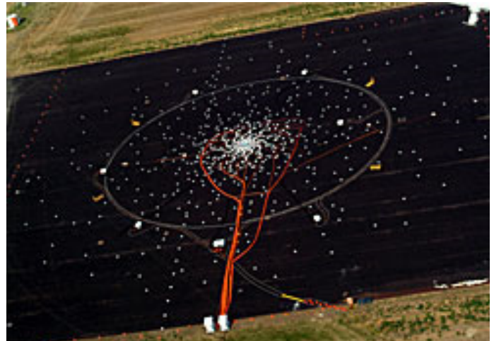
FIG 19 By using a PXI architecture configured for mass synchronization across multiple chassis, Boeing synchronized more than 600 ground-based microphones for data acquisition while reducing cabling and cost per channel.
